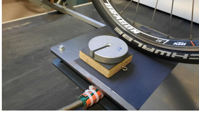
Figure 5.2: Experiment set-up for measuring the coefficients of friction
